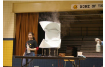
A 55-gallon drum imploded after water vapor was sealed inside to cool.
